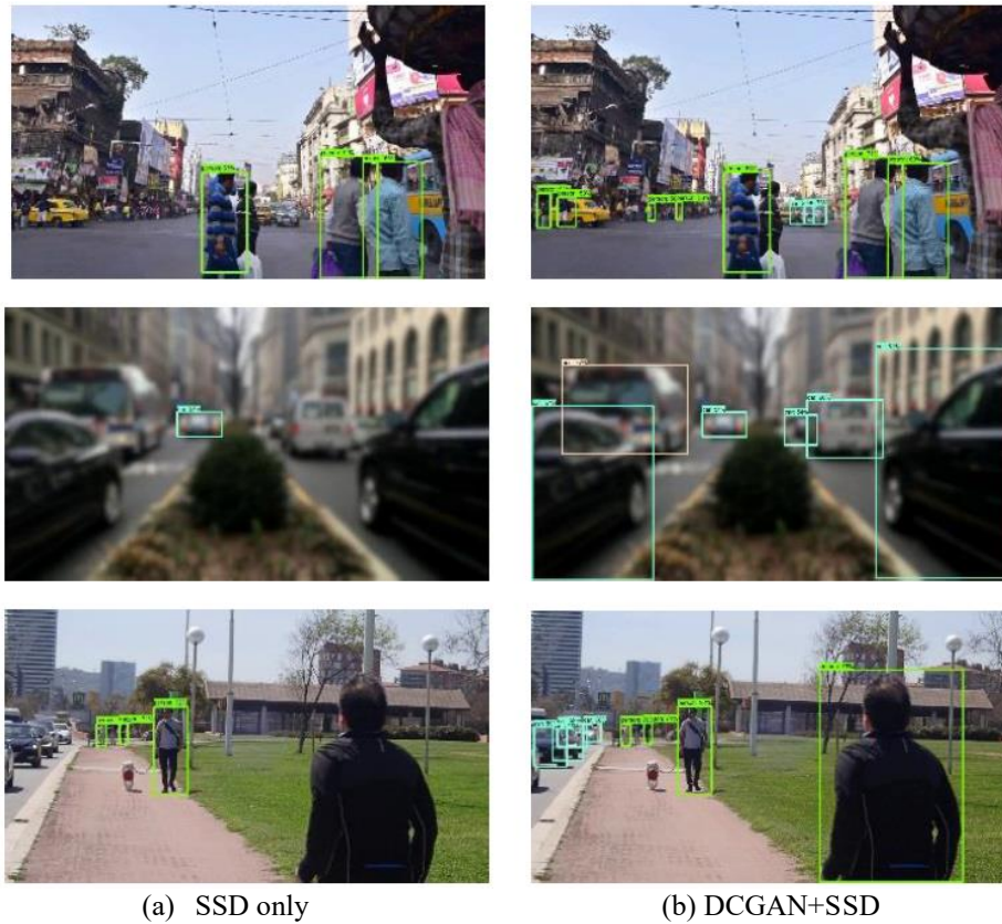
Fig.3. Detection examples for comparison. a) Results with SSD only; b) Results with DCGAN+SSD.
