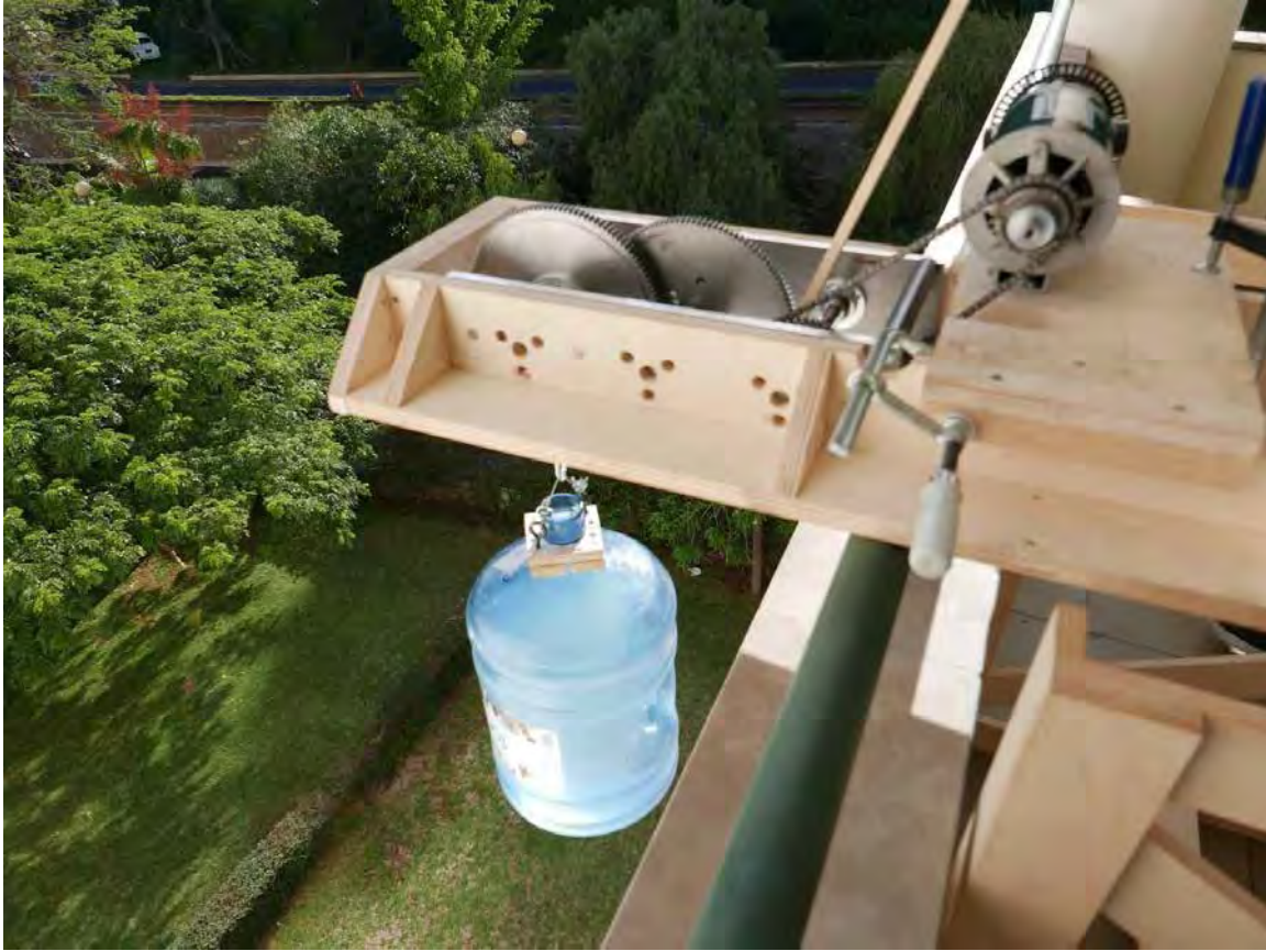
Fig. 2 Detail of the gravity battery mechanism and weight
