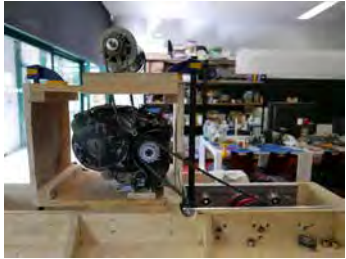
Image 5: Challenge #7: The gravity battery, an alternative form of energy generation we propose as an instance of Reconstrained Design. ©The authors
