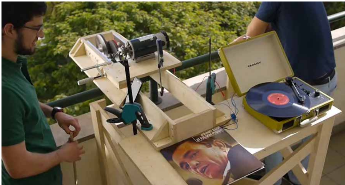
Fig. 1 Gravity battery powering an out-of-the-box record player: https://vimeo.com/202043363
