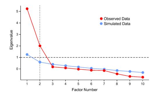
*Figure 3.3* Scree plot including parallel analysis. Factors 1-2 have larger eigenvalues based on the observed data than when based on simulated data
