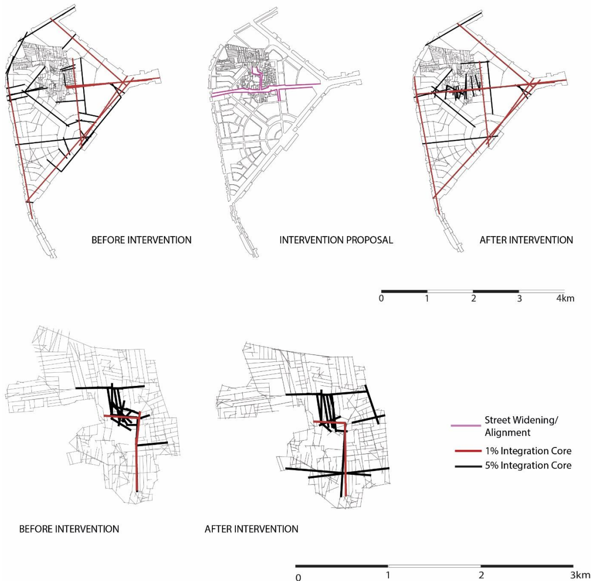
Figure 9: Mit Uqba and its surrounding planned settlement Mohandisseen before and after intervention (top) and Mit Uqba's syntactic structure before and after intervention (bottom)
