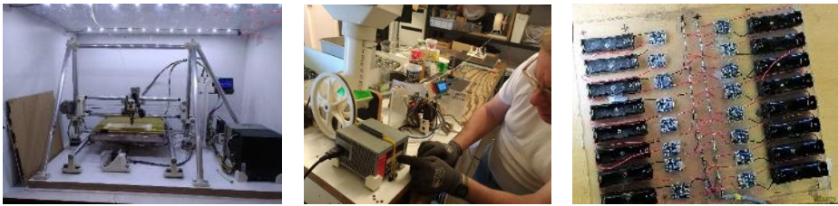
Fig. 2: from left to right: a 3D printer, 3D printer filament extruder, and battery charging board, all created from recyclable materials at the centre.
