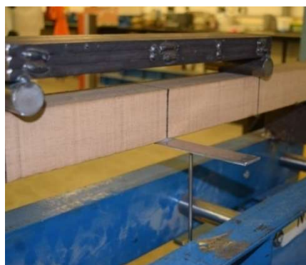
Figure 2. Measurement of vertical deflection at mid-span using LVDT.
