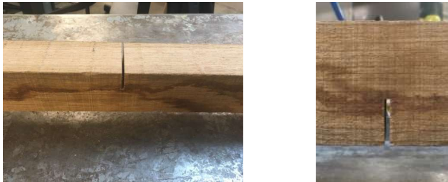
Figure 3. Damaged beam specimens (cut dimensions: 20 x 67 mm).
