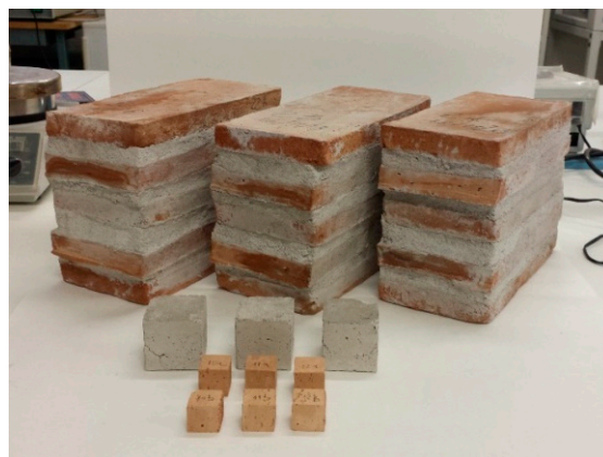
Figure 7. Different typologies of tested specimens (letter designation: Br = Brick, Mo= Mortar, Ma = Masonry).
