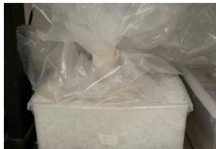
Figure 10. Masonry specimens buried in the refrigerating mixture.
