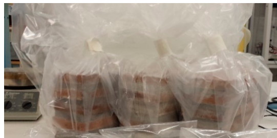
Figure 9. Masonry specimens inside the polyethylene (PE) bags.
