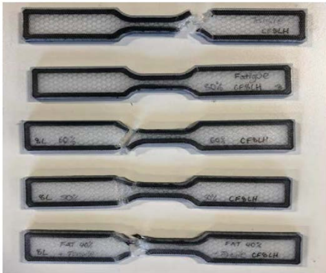
Fig. 4. Fatigue testing and failed samples
