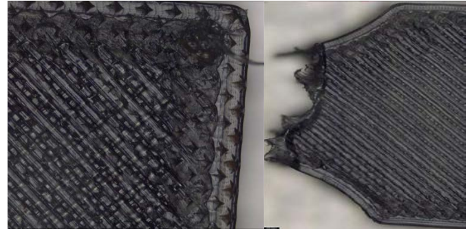
Figure 8 - Optical microscope pictures of carbon reinforcement and failed section
