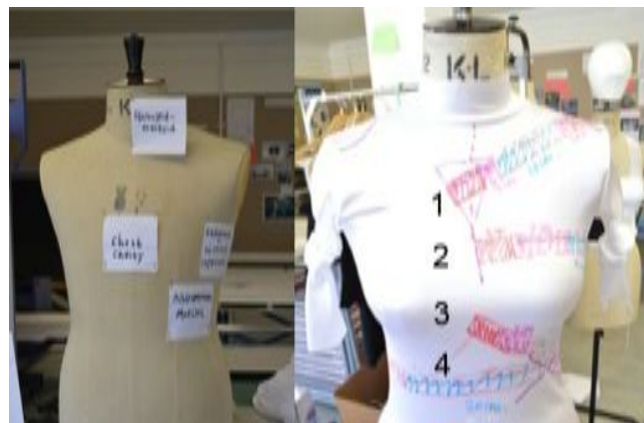
Figure 2 – Positioning the sensors
