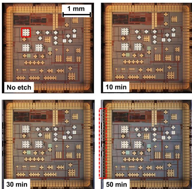
Fig. 11. Optical images of a CMOS ISFET chip, with patterned spray-coated photoresist prior etching and 10, 30 and 50 min after  $O_2$  plasma etching (dashed area shows some of the bonding pads that are partially exposed).
