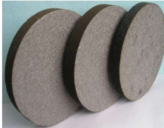
Fig. 3 Test samples of sintered fibrous metal
