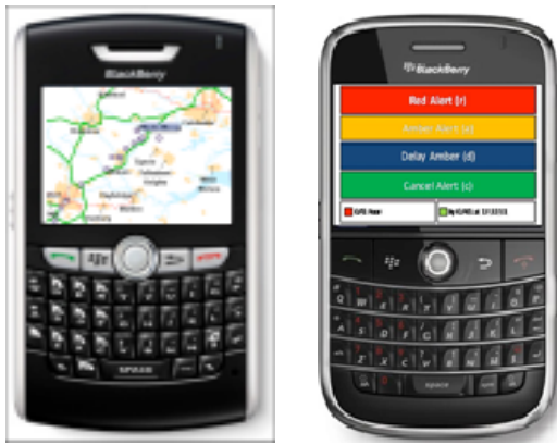
Figure 3. A BlackBerry 8800 displaying a typical location map (left), and an example of the Alert Client: ‘Red Alert, Amber Alert, Delay Amber, Cancel Alert’ (right).
