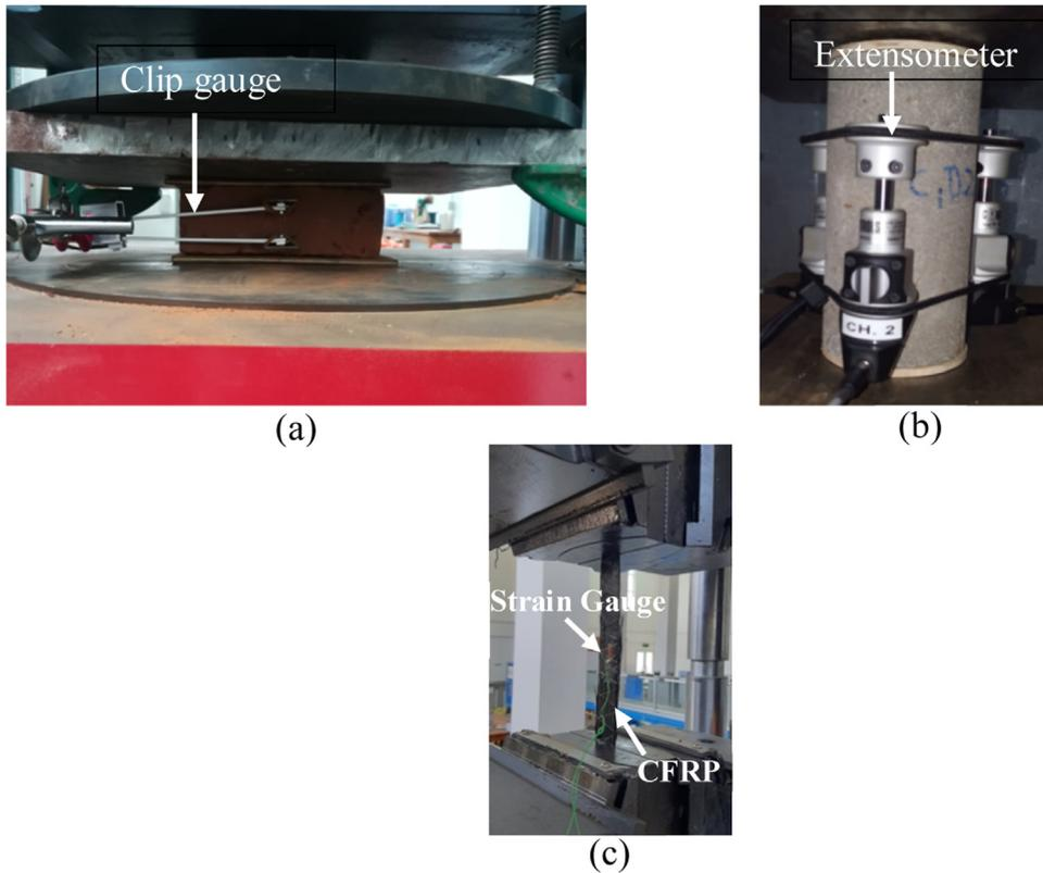
**Fig. 1.** Material characterisation (a) brick compression testing (b) mortar compression testing and (c) tensile testing of CFRP.
