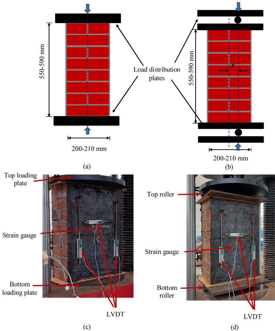
Fig. 3. (a) Diagram of concentric loading set-up (b) Diagram of eccentric loading set-up (c) Concentric loading testing and (d) Eccentric loading testing.
