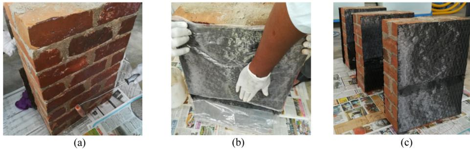
**Fig. 2.** CFRP application processes on the masonry wallettes (a) application of epoxy resin on masonry (b) pasting of CFRP sheets on masonry surface and (c) CFRP strengthened masonry.
