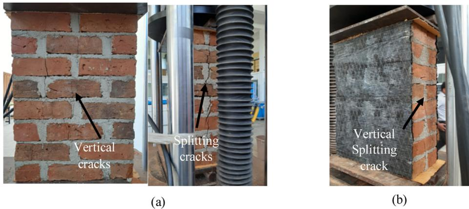
Fig. 5. Failure patterns of eccentric loaded wallettes (a) Un-strengthened and (b) Strengthened.
