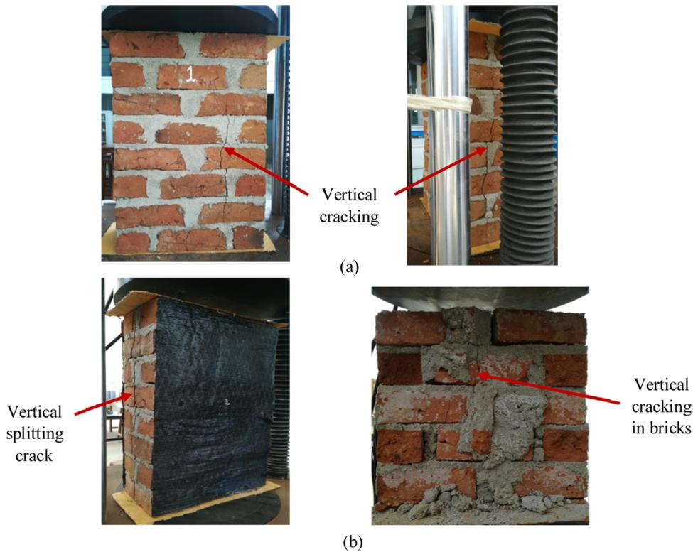
**Fig. 4.** Failure patterns of concentric loaded wallettes (a) Un-strengthened and (b) Strengthened.
