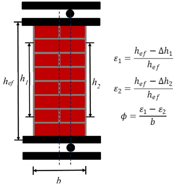
Fig. 7. Scheme for the calculation of the curvature.
