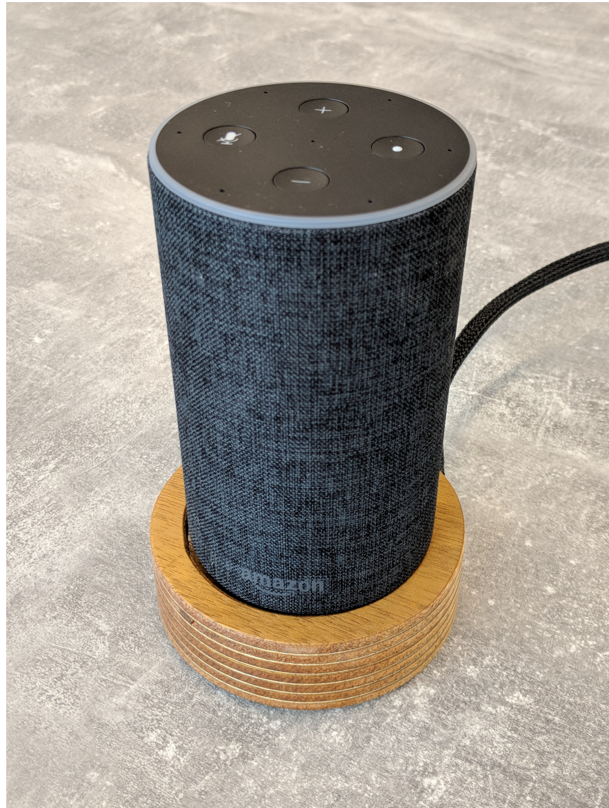
Figure G.1: The two parts that comprise Spkr: Part A: Raspberry Pi computer inside wooden base (bottom). Part B: Amazon Echo speaker (top)
