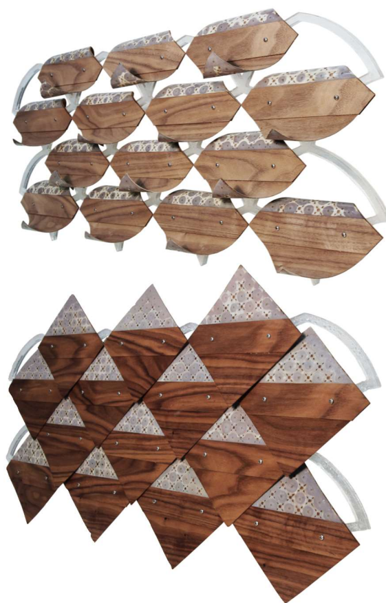
Figure 3. Prototype hygromorphic cladding panel comprising walnut veneer bonded to laser perforated fibre glass, with apertures which are open when dry (top) and closed when wet (bottom). Image by Artem Holstov.
