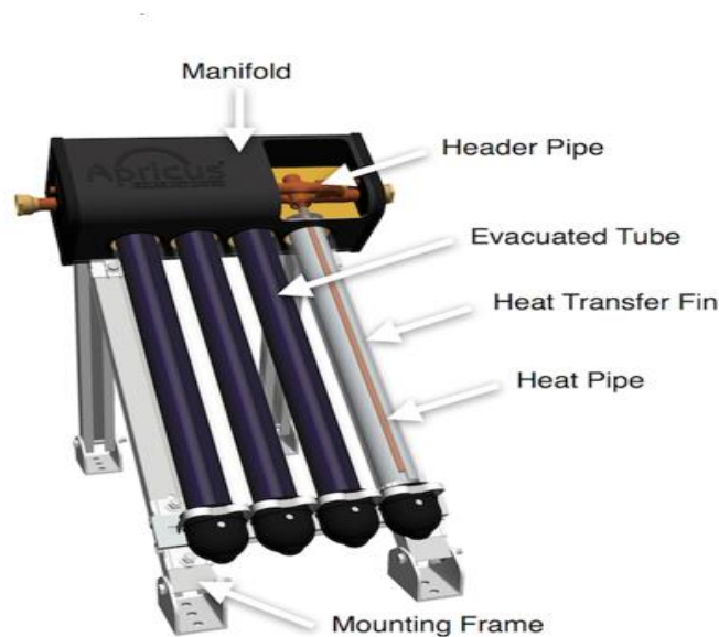
Figure 2.5 The schematic of the ETC [87]
