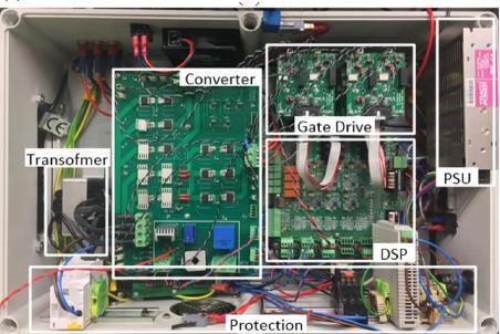
FIGURE 9 Photos (a) test bench; (b) prototype converter
