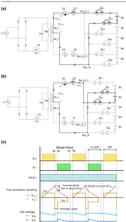
**FIGURE 5** Equivalent circuit for equalisation from  $B_1$  to  $B_2$  for inductor: (a) charging period; (b) discharging period; (c) key operational waveforms
