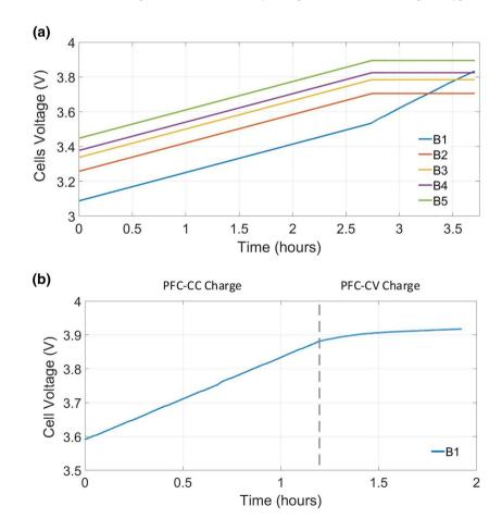
**FIGURE 11** Cells voltages during charging under (a) open-loop control; (b) power factor control-CC control
