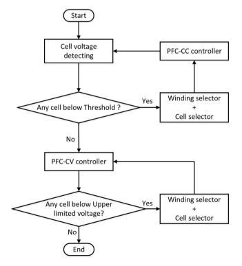
FIGURE 7 Flow chart of the proposed control algorithm
