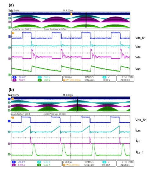
FIGURE 10 Experimental results when charging five cells: (a) voltage waveforms; (b) current waveforms
