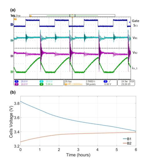
**FIGURE 13** Waveforms of voltage equalisation from  $B_1$  to  $B_2$ : (a) voltage and current in the converter; (b) cells voltage
