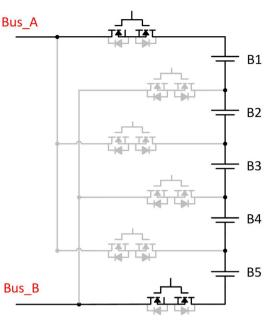
FIGURE 3 Examples of battery strings as sink cells
