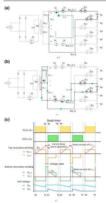
**FIGURE 4** Equalisation from B1 to B3: (a) magnetising period; (b) demagnetising period; (c) key operational waveforms
