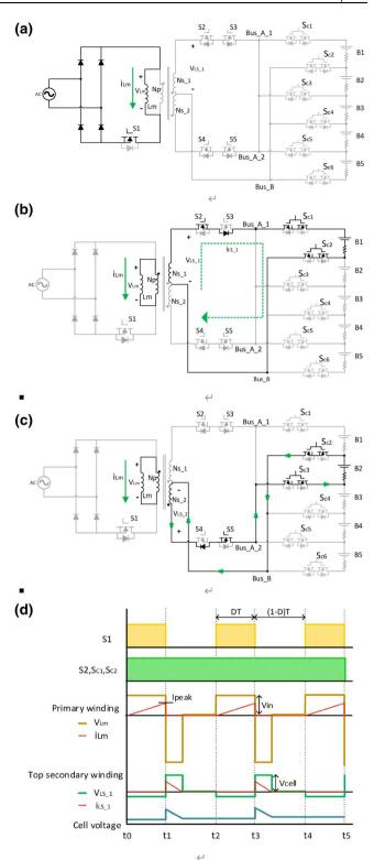
**FIGURE 2** Grid charging: (a) magnetising period; (b) charging for odd-numbered cells; (c) charging for even-numbered cells (d) operational waveforms for charging B1
