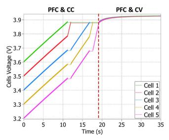
**FIGURE 8** Simulation results of battery charging with power factor control-CC-CV controller
