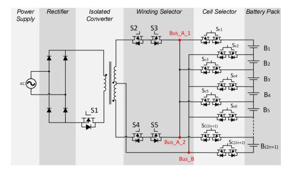
FIGURE 1 Proposed multi-functional battery charger integrated with voltage equalisation in (2n+1) battery cells
