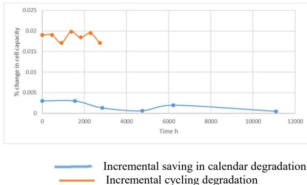
Fig. 5 Incremental cycling degradation vs. calendar degradation
