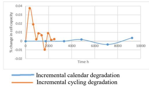
Fig. 3: Incremental cycling degradation vs. incremental calendar degradation
