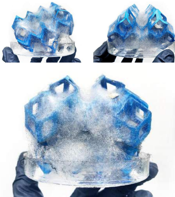
Fig. 14. Mycelium grown on paper-based origami scaffold coated with Agar-Agar
