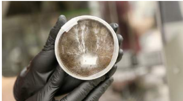
Fig. 17. Mycelia growing on Martian regolith simulant.
