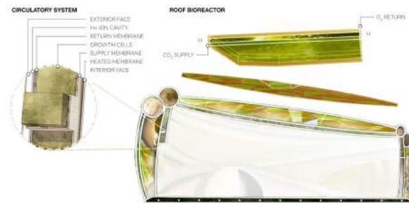
Fig. 3. Habitat acting as an integral bioreactor, redhouse studio
