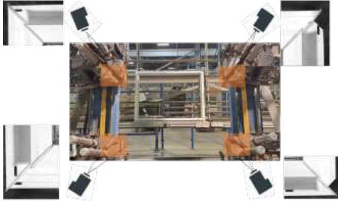
Figure 2. Illustration of the proposed inspection system on a VSM Sturtz four-point automated welding machine.
