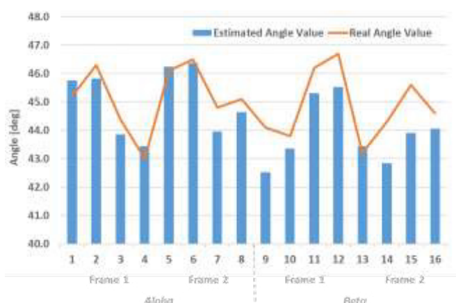
Figure 6. Inspection results vs. angle measurements for the test window frames.
