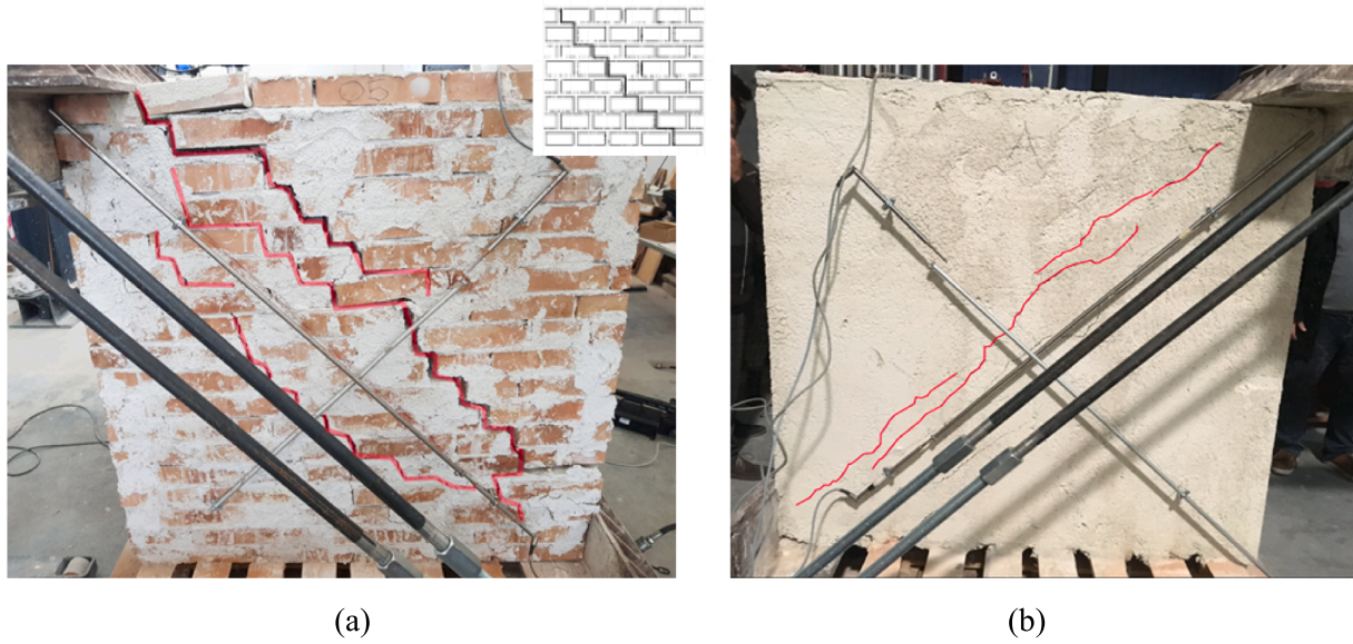
Fig. 3. Failure mode of wall panels tested in the first phase of the experimental work: (a) unreinforced specimens, (b) reinforced with FRCM (rigid GFRP grid embedded into a mortar coating).
