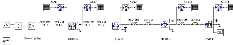
Fig. 5. The VPI simulation setups for four-hop routing.
