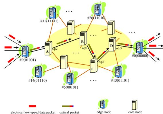
Fig. 1. An optical core network with 32 edge nodes.
