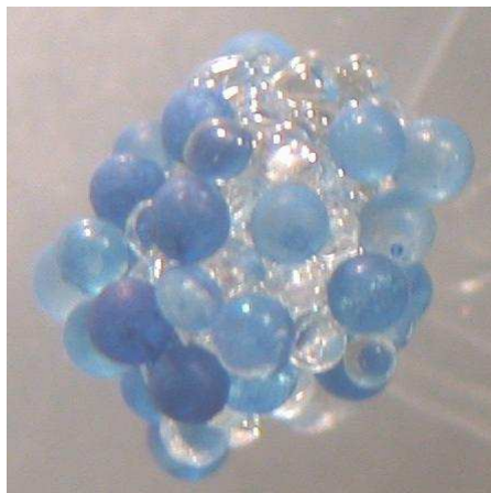
Figure 3 Aggregate of blue hydrophobic spheres surrounding transparent hydrophilic spheres after the formation of clumps during evaporation.
