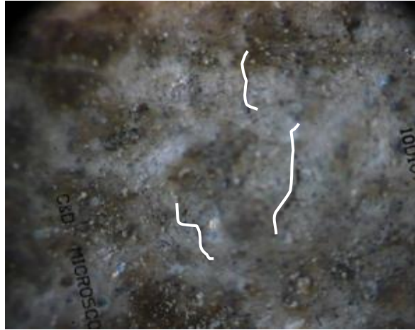
Figure 6 Shrinkage cracking on cigarette filter concrete
