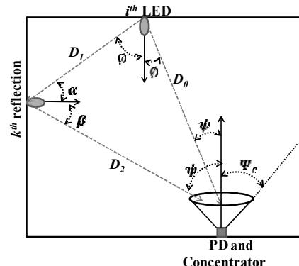
Fig. 2 Lighting and received communications power model
