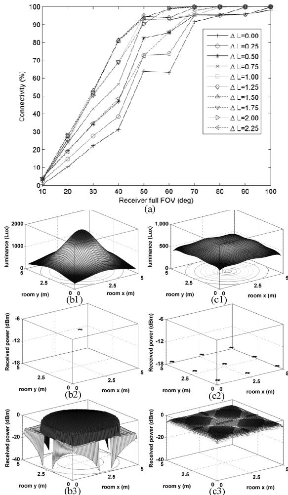
Fig. 4 (a) VLC connectivity percentage throughout the RP; (b1) luminance footprint  $\Delta L=0$  m, (b2) received power  $FOV_{Rx}$  (full)= $10^\circ$ , (b3) Received power  $FOV_{Rx}$  (full)= $100^\circ$ ; (c1) luminance footprint  $\Delta L=2.25$  m, (c2) received power  $FOV_{Rx}$  (full)= $10^\circ$ , (c3) received power  $FOV_{Rx}$  (full)= $100^\circ$ .
