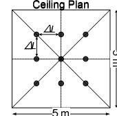
Fig. 1 Ceiling plan for the LED array layout (LED array = dark spots)
