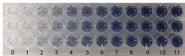
Fig. 1 Reaction of OPA reagent with ammonia (concentration of \text{NH}_4\text{Cl} standard solution in mM indicated as number) after dilution with DMSO.
