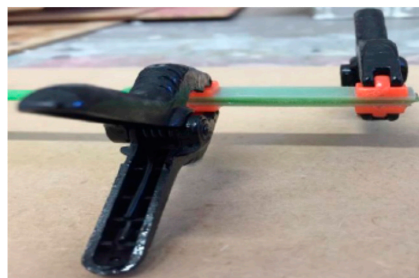
Figure 7. Detail of the epoxy tabs glued at both ends of the specimens.
