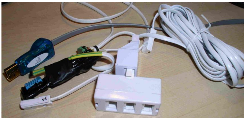
Figure 4.32. Humidity and temperature sensor network.
