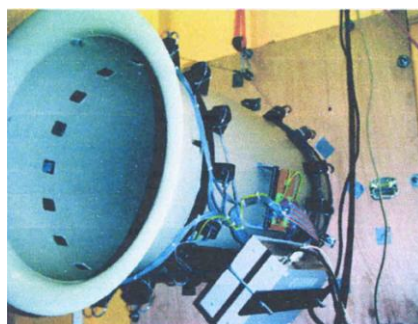
Figure 2.3. Acoustical ventilation rate sensor for naturally ventilated buildings by Buggenhout et al. (Source: Buggenhout et al. , [22] (p. 195))
