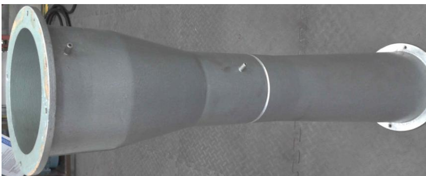
Figure 4.36. Short-form Venturi used in experiments.
