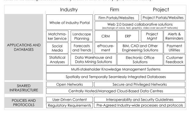
Fig. 3. Components of the Composite ICT Landscape for the Building Construction Industry
