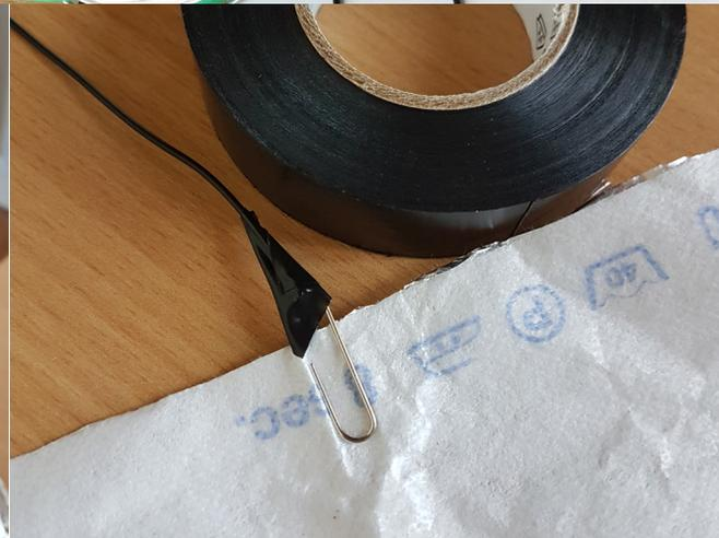
**STEP8:** Use a bit of insulating tape to protect the soldered connection from bending and breaking.
