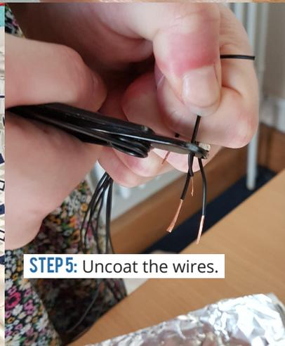
**STEP5:** Uncoat the wires.
