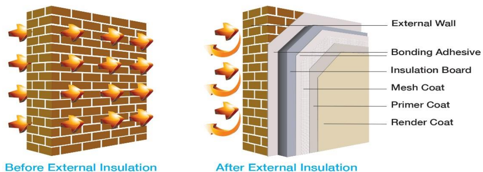
Figure 2.23 Before and after external solid wall insulation (Heat-Insulation, 2018)
