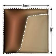
Fig. 1. Optical image of a  $3 \times 3$  mm silicon chip with spin-coated photoresist showing significant edge bead (dashed line area).
