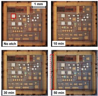
Fig. 11. Optical images of a CMOS ISFET chip, with patterned spray-coated photoresist prior etching and 10, 30 and 50 min after O<sub>2</sub> plasma etching (dashed area shows some of the bonding pads that are partially exposed).
