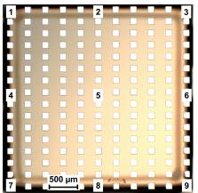
Fig. 6. Optical image of spray-coated chip after photoresist development. Numbers indicate approximate locations where the thickness of the photoresist has been measured using reflectometry.
