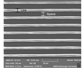
Fig. 9. SEM image of  $5\mu m$  wide dense 1:1 line and space features patterned on ~9  $\mu m$  thick spray-coated photoresist.
