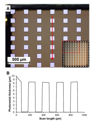
Fig. 7. (A) Optical image of a section of the spray-coated chip, with the arrow indicating the direction of a profilometry scan. (B) Surface profile trace of the above scan, showing the photoresist thickness variation.
