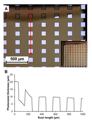
Fig. 4. (A) Optical image of a section of the spin-coated chip, with the arrow indicating the direction of a profilometry scan. (B) Surface profile trace of the above scan, showing the photoresist thickness variation.
