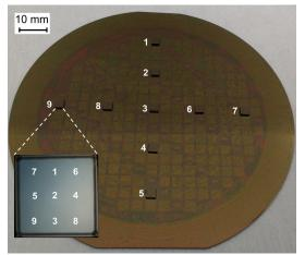
Fig. 8. Photograph of carrier wafer comprising multiple chips to investigate the on-chip spray-coated photoresist thickness across a wafer. The blown-up optical image of one the chips shows the approximate measured positions for each chip.
