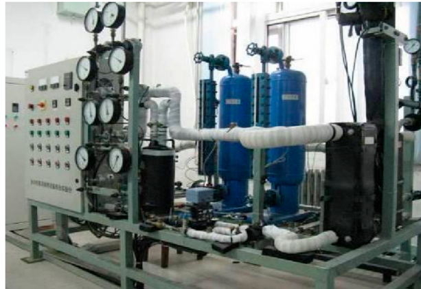
Figure 5. The test-bed of a compression refrigeration system.
