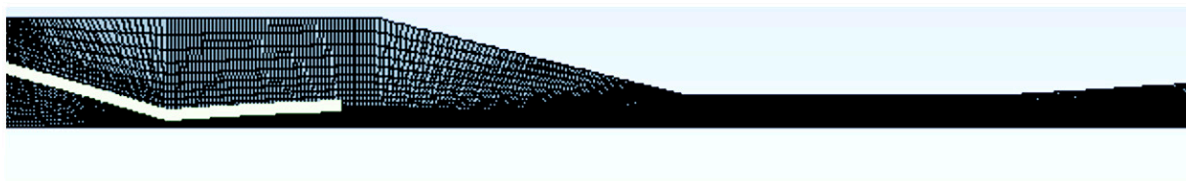
Figure 5. Structured meshing for AG1 with 9940 elements for axisymmetric modeling.
