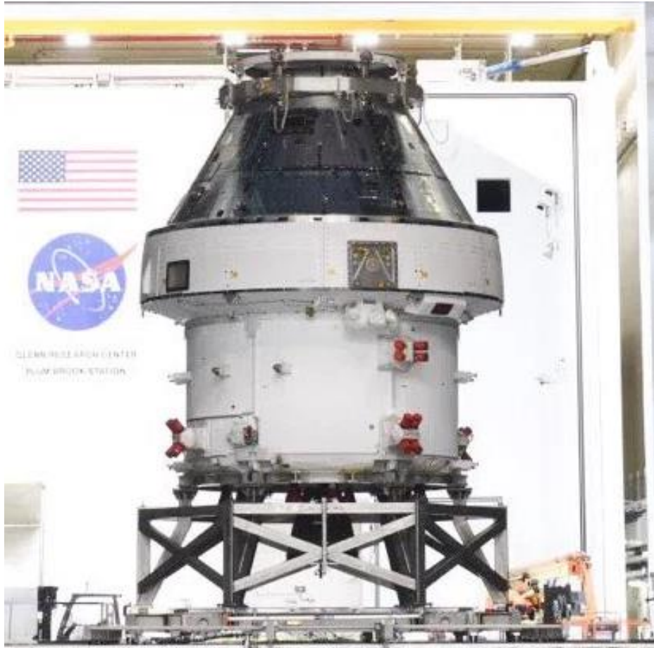
Figure 1.1 The Orion MPCV crew module (top) with European Service Module (base) attachment (Etherington, 2020)
