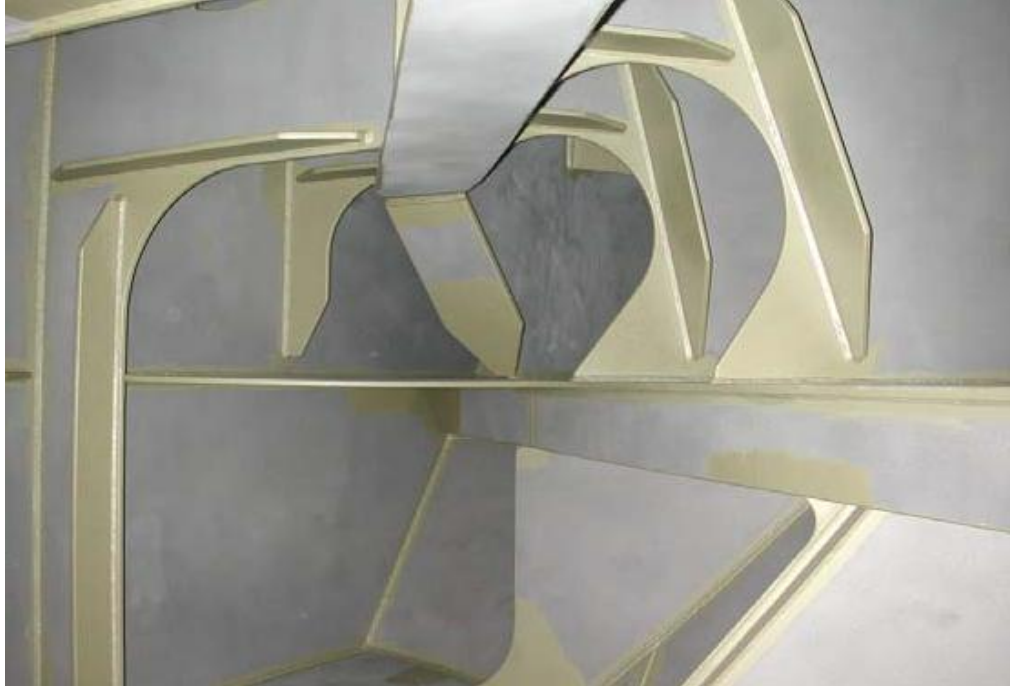
Figure 23 Typical critical areas striped coated in a WBT
