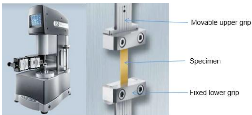
Figure 41 Tension fixture of RSA G2 rheometer analyser
