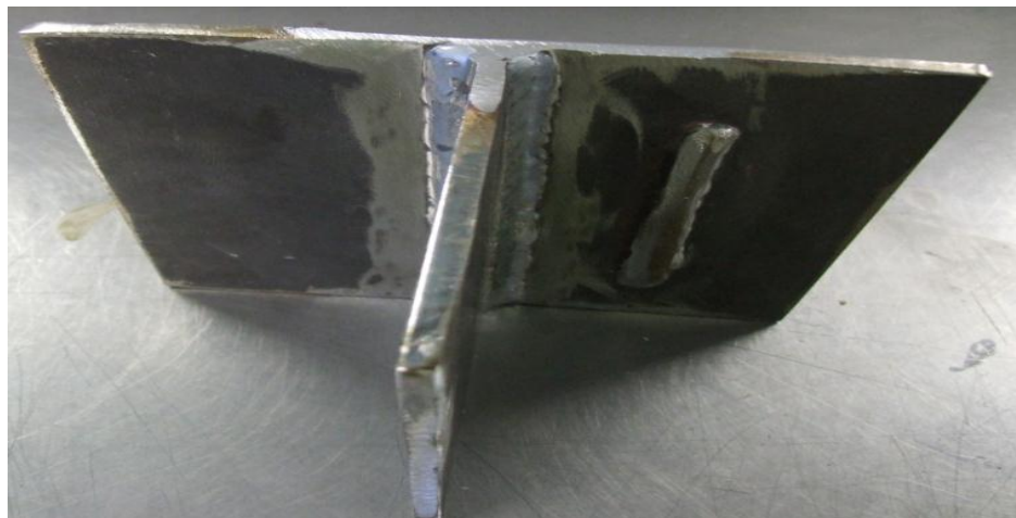
Figure 21 Pictorial view of the "as received" bare T sectional substrate
