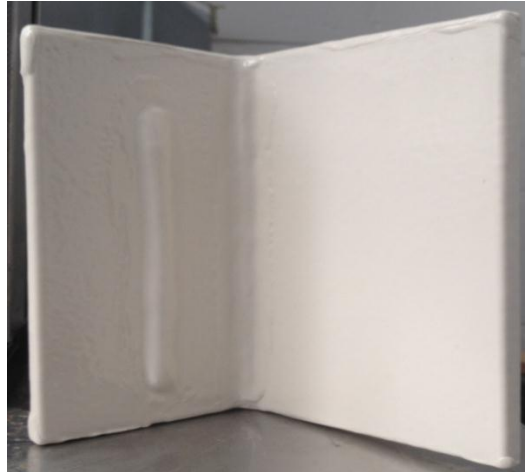
Figure 29 Coated T specimen
