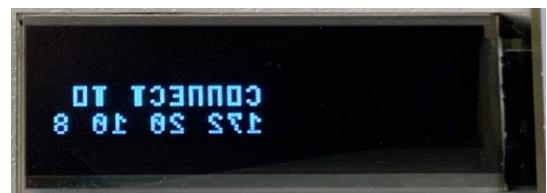
FIGURE 5. Example of custom font type displayed on the micro-LCD (Note the text is reversed.)
