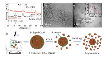
**Figure 2.** Synthesis and structural characterizations of the catalysts. (a) XRD patterns of B-doped Cu<sub>2</sub>O catalysts before and after CO<sub>2</sub>R. (b) TEM and (c) HRTEM images of fragmented Cu catalysts after CO<sub>2</sub>R. The inset image in (c) is the statistic of particle size. (d) Schematic illustration of the structural evolution of fragmented Cu catalyst.
