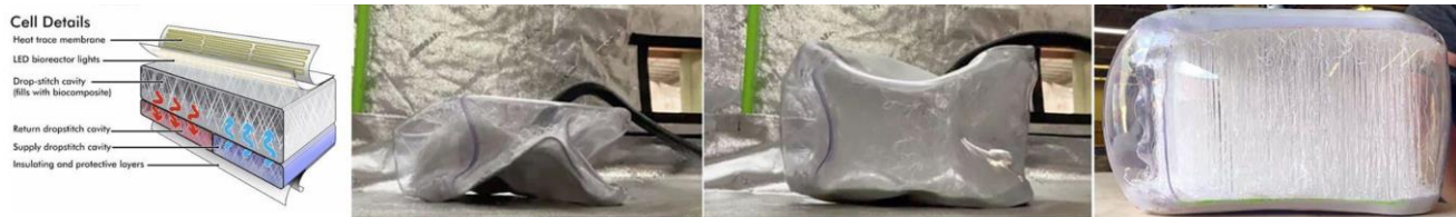
Fig. 7. Drop-stitch technology, inflatable prototype, redhouse studio
