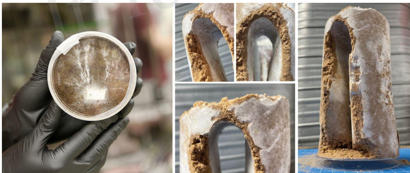
Fig. 8. Mycelia growing on Martian regolith simulant, Sand structures
