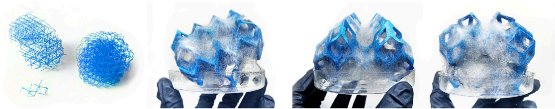
FIGURE 6 Scaffoldings. Example of lattice from Solus printer available in Rothschild's lab, mycelium growing on paper-based origami scaffold coated with nutrients and agar.
