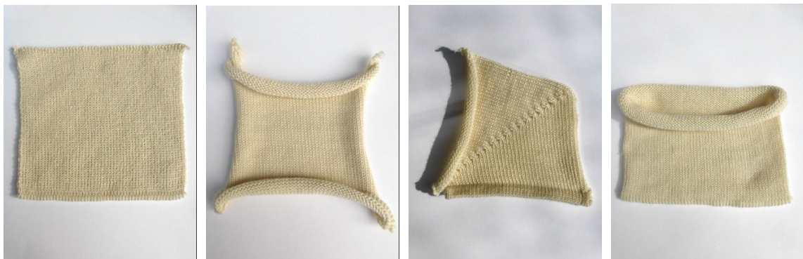
Figure 2: Knitted Fabric Structures: left to right rib and plain (stitches formed in opposing directions on alternate courses), partial knit (increasing and decreasing stitches), tubular (stitches formed spirally in the round).
