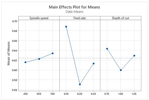
Fig. 4: Main effects plot for GRG (PKO lubricant)
