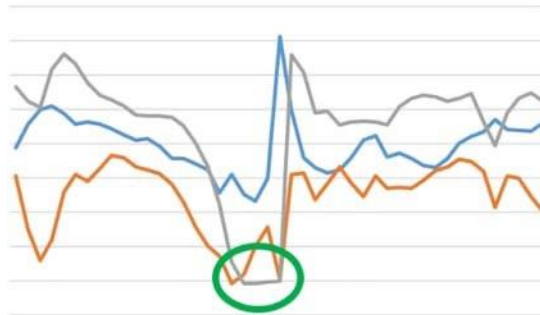
Figure 5. Tri-axial accelerometer signals with grey trace/signal clipped (green circle) and so hasn't adequately captured (gait) task
