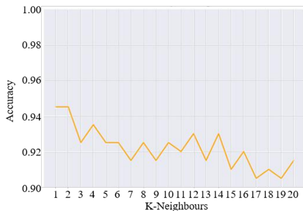
Figure 4.5: Classification accuracy on the test dataset portion for the k-NN algorithm used, with varied k-neighbour values.
