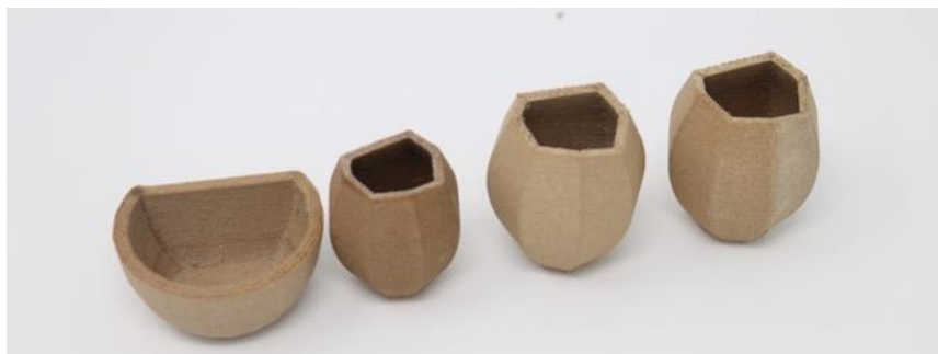
Figure 4.9-15 Explorations of the form in relation to the size of the electronic components. 3D printing with wood filament. approx.3cmx5cm.
