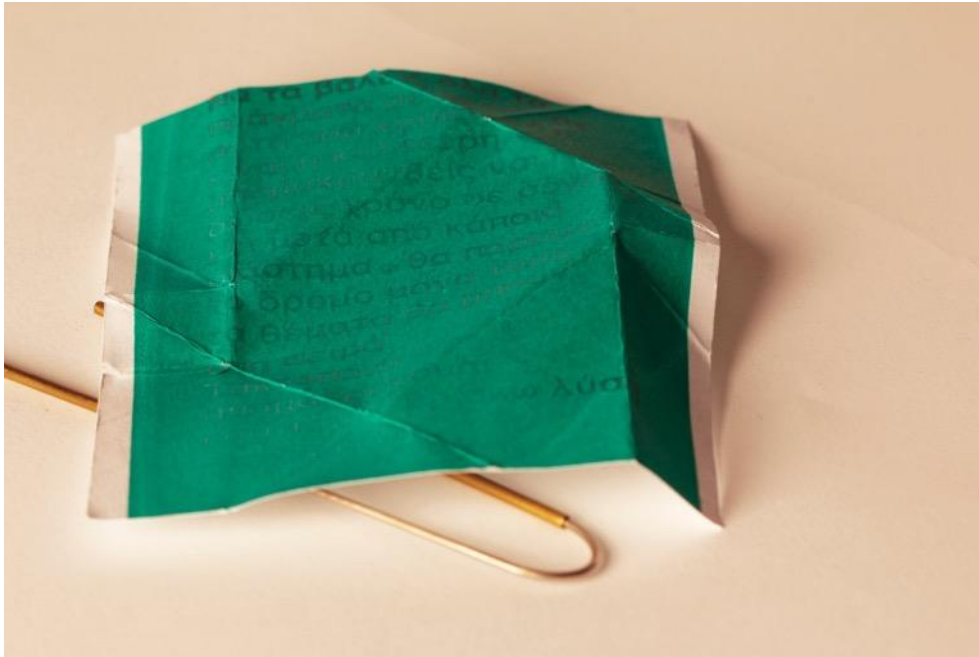
Figure 4.3-8 Hide and Seek Piece. The text slowly disappears as the temperature rises over 27°C. The picture was taken in Greece during the summer.
