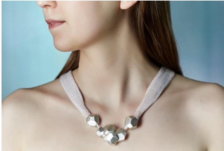
Figure 2.2-1 Smart Heart cardiac monitor necklace by Leah Heiss, 2016 in collaboration with St. Vincent’s Hospital Melbourne, RMIT University, and the Nossal Institute for Global Health; 3d printed parts, conductive threads, sensors.
