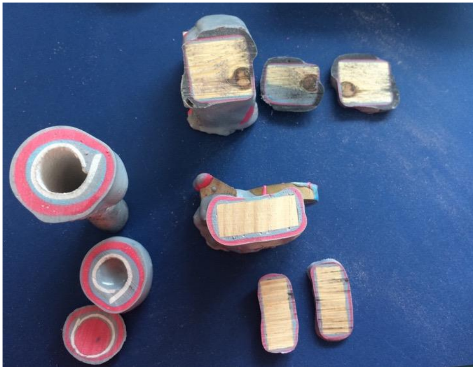
Figure 4.9-16 Initial Explorations. Dipping pieces into layers of coloured resin.
