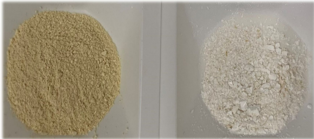
Figure 22. Crude mycoprotein (left) and \beta -glucan fraction (right) obtained in the alkaline extraction protocol.
