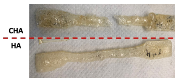
Figure 128: Initial dogbones produced from both CHA and HA-based DER 332 polymer formulations crosslinked with 40% DEA consumption by diboronic ester 6.
