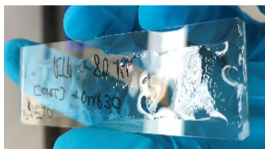
Figure 115: Photo of polymer film B2 after room temperature cure for 24 hours followed by a thermal cure at 80 °C for 16 hours.
