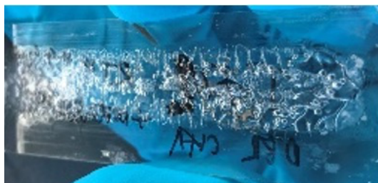
Figure 117: Picture of fractured and aerated film B3 film with 100% equivalence of diboronic crosslinks.
