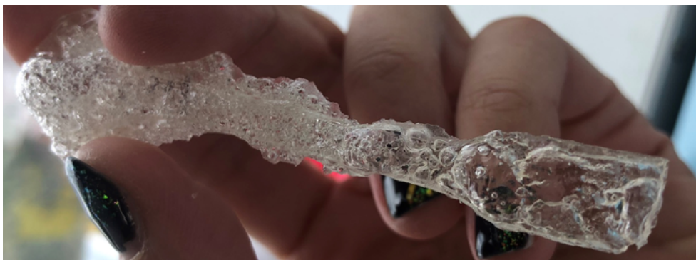
Figure 131: post-thermal cure, under vacuum, HA-E1(DEA-5)-D40 polymer.
