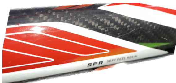
Figure 6: Visible woven carbon fibre (Black) in a 35% carbon composite hockey stick.
