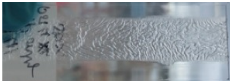
Figure 126: Polymer HA-E1(DEA-5) with 40% diboronic ester (D40) consumed DEA groups after draw-down onto glass slide and cured at room temperature for 24 hours followed by a thermal cure at 80 °C.
