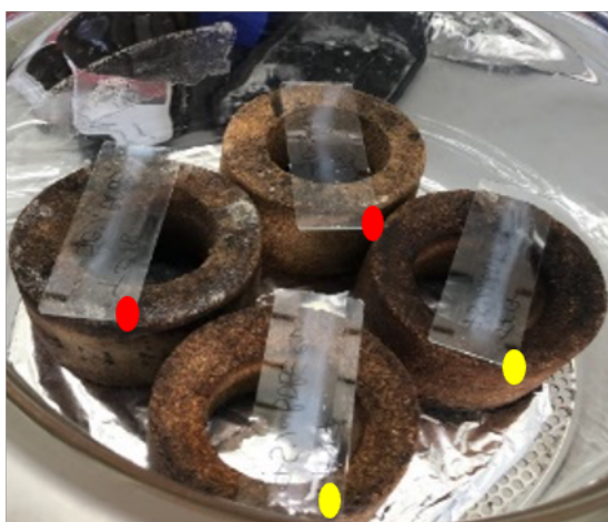
Figure 118: CHA films with 75% diboronic ester content (yellow) and 50% boronic ester content (red) after a room temperature cure in a desiccator.
