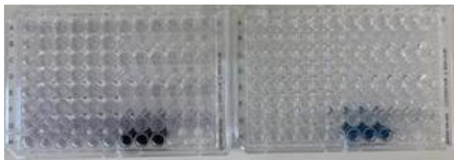
Figure 3.8 Microtiter plate with positive control. On the left side plate is the neat standard solutions of \text{NH}_4\text{Cl} , while on the right plate is the diluted in DMSO to allow concentration determination by UV/visible spectroscopy.
