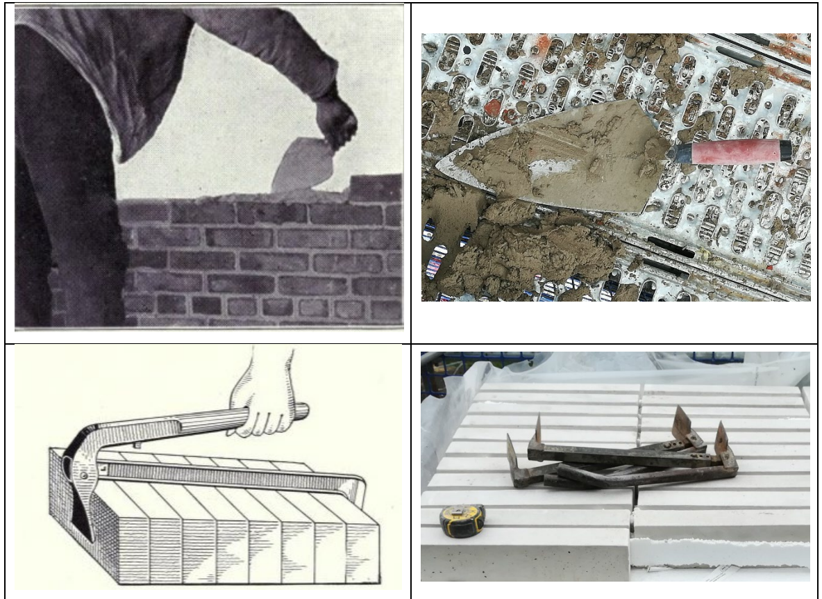
Figure 2.1 Top: Trowel, Bottom: Brick clamp (Left: Gilbreth (1909, pp. 8&118), Right: Photos taken by Orsolya Bokor in 2019)
