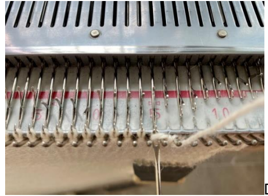
Figure 5:3 Step 2: Knit the body of the sample in the chosen pattern. Bind off the knit and take off the machine.
