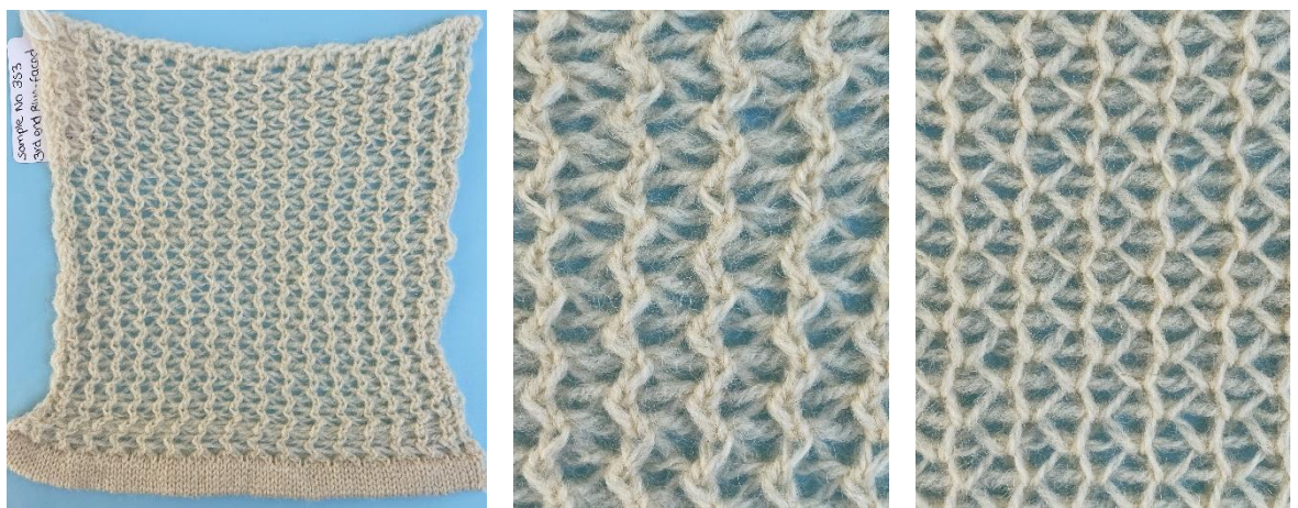
Figure 7:8 Sample 353, A 3x1 ladder structure, manipulated with racked look pick up technique. 13
