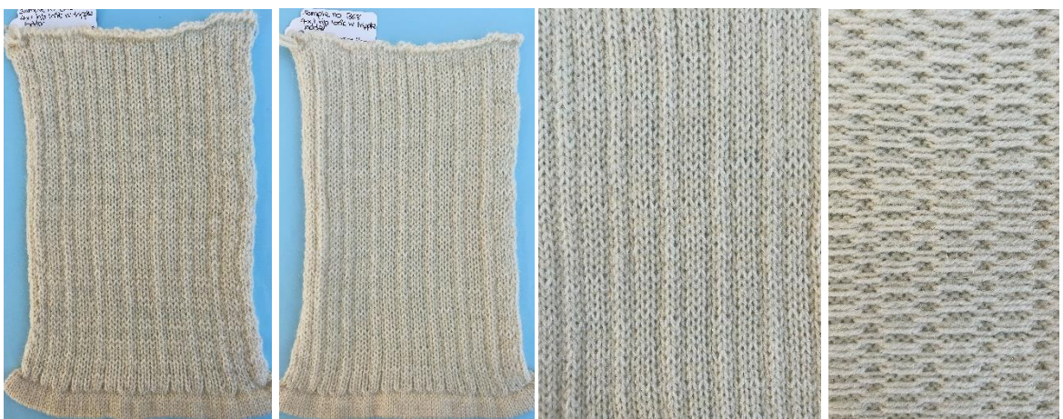
Figure 7:18 Samples 366 & 368, 4x1 rib-look float jacquard's with a triple ladder structure.
