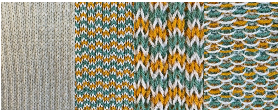
Figure 7:58 Sample 371 is a 4x1 rib-look with three yarn types with a double-double* ladder structure. WFW in feeder A, BFL2/ DH interchange through feeder B.
