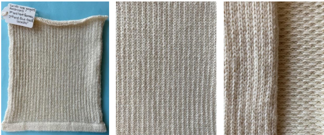
Figure 7:27 Sample 307, a 2x1 rib-look float jacquard structure.
