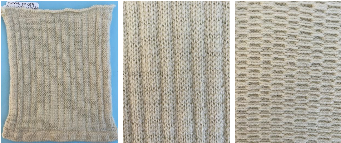
Figure 7:16 Sample 369, a 4x1 rib-look float jacquard with single ladder structure.
