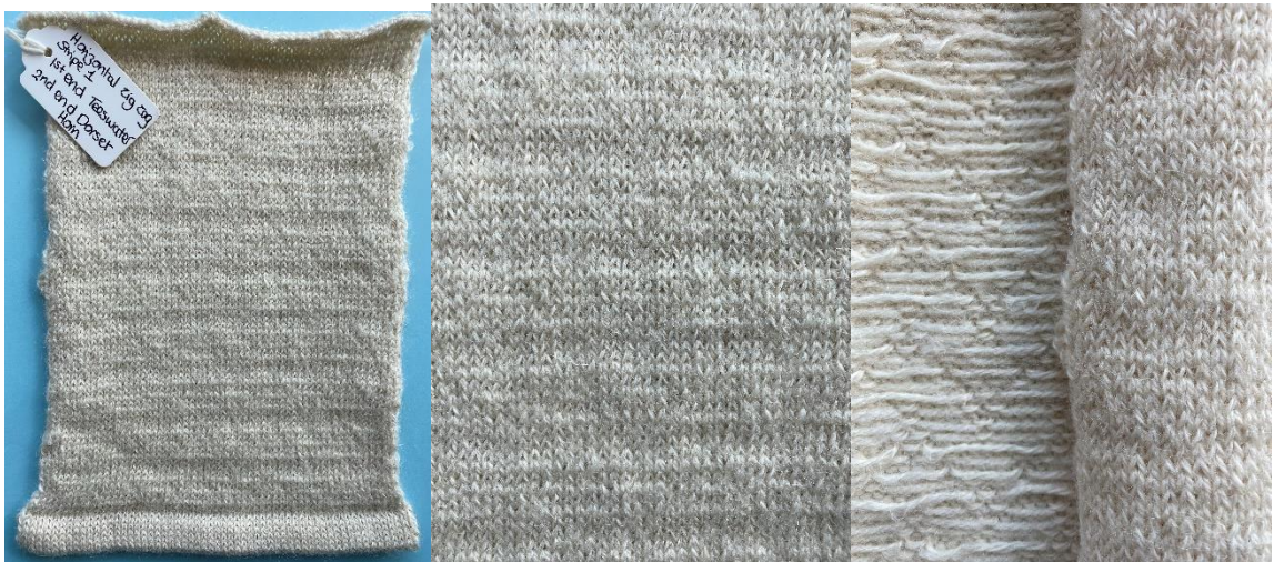
Figure 7:26 Sample 104, horizontal zigzag 1 float jacquard structure in Tees/DH
