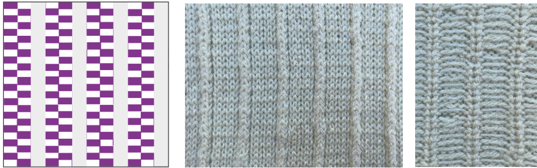
Figure 6:12 Sample 273 is a 2x1 rib look tuck jacquard structure with a double ladder. The images show the front and back of the knit. Sample 264 was knitted in the same structure.
