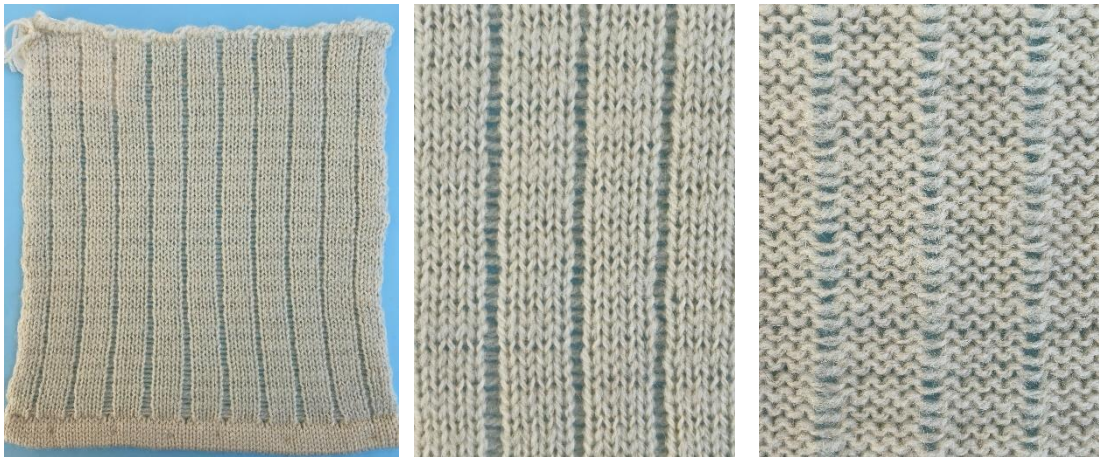
Figure 7:4 A 1x1 course stripe structure with a single ladder repeat throughout.
