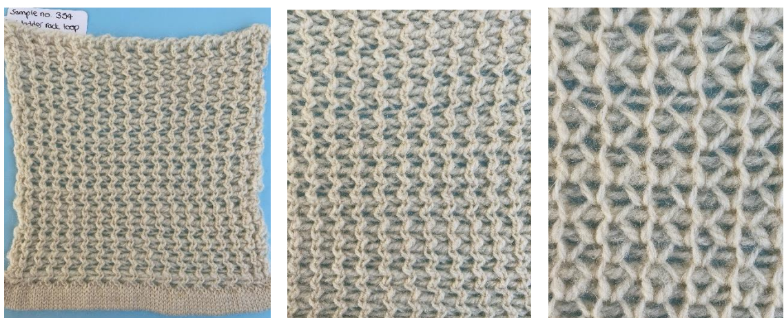
Figure 7:8 Sample 353, A 3x1 ladder structure, manipulated with racked look pick up technique. 13
