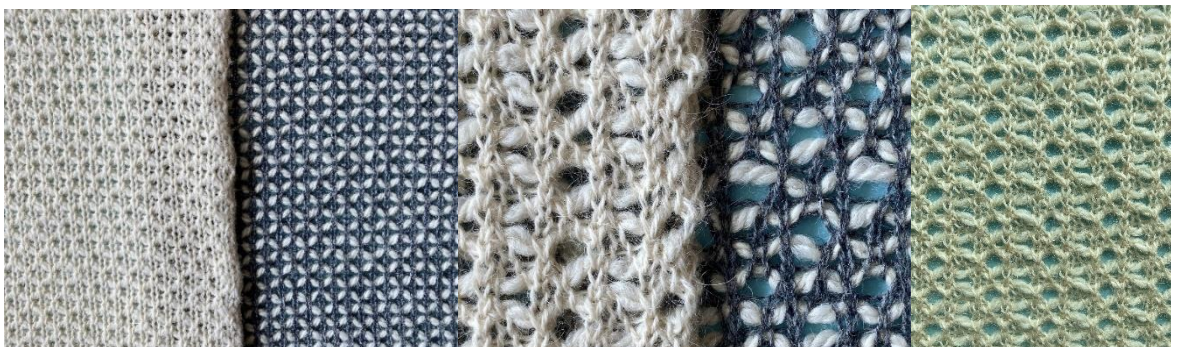
Figure 6:31 Details of sample 58 (1x1 inlay) and sample 21 (1x1 Inlay with pointelle). The images show the front and reverse of the swatch in ecru and colour to visualise how the yarns have combined together.
