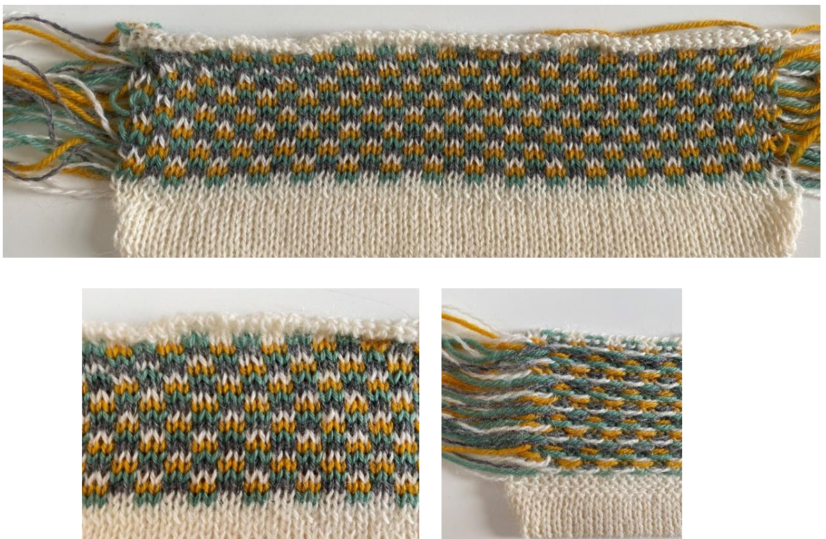
Figure 7:42 The images above demonstrate how a 2x1 rib-look pattern changes the yarn type on every course. (This is represented by four colours.)
