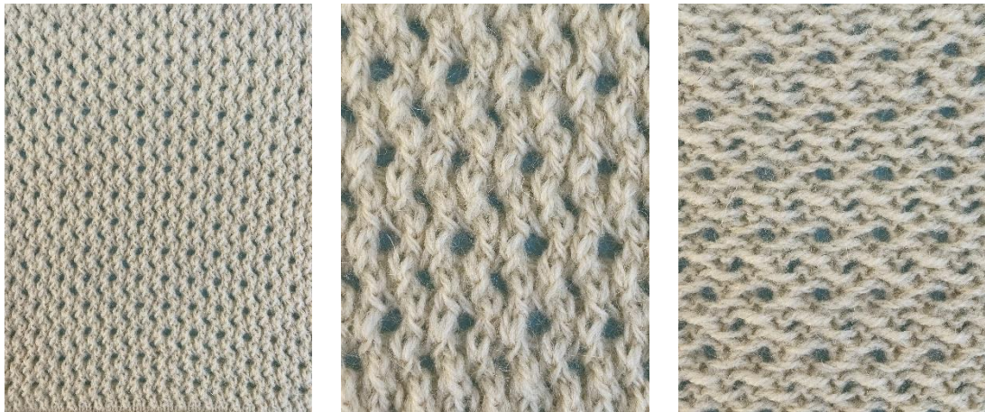
Figure 7:51 Samples 380 & 382 three and four yarn blend variations of a 2x1 float jacquard pattern with pointelle.
