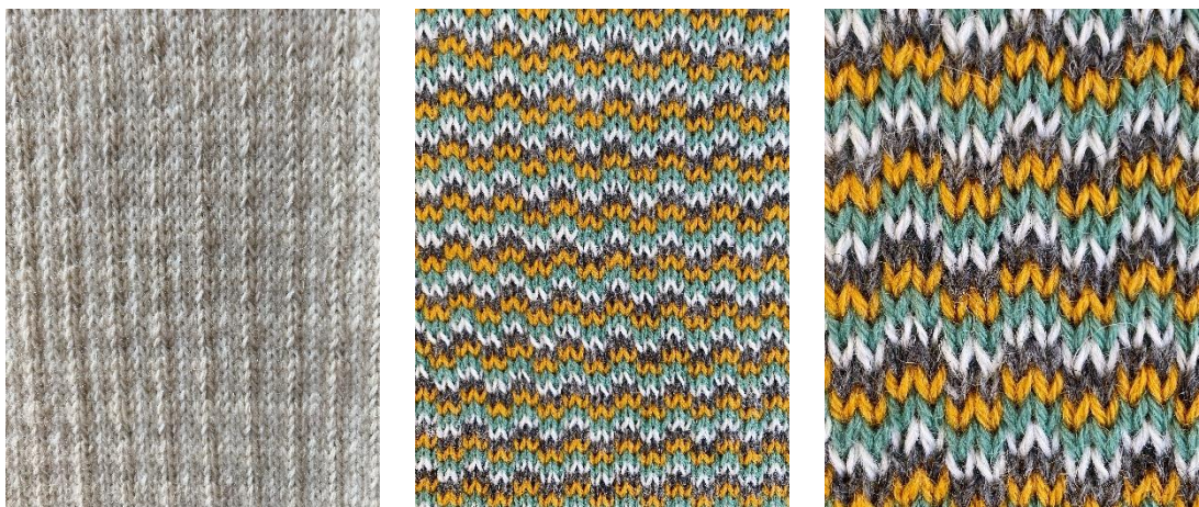
Figure 7:49 Sample 311 a 2x1 rib-look structure in a four yarn blend (DH, KR, BFL2, Teeswater) in ecru and colour.
