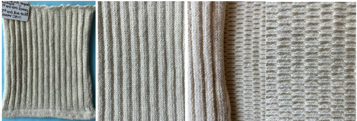
Figure 7:23 Sample 137 4x1 rib-look float jacquard sample, demonstrating rib-look structure.
