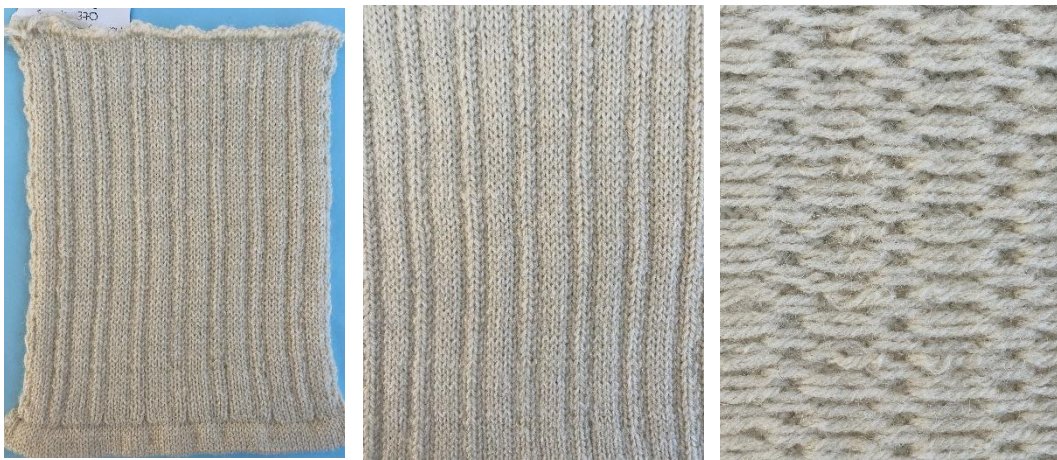
Figure 7:17 Sample 370, a 4x1 rib-look float jacquard with a double ladder structure.
