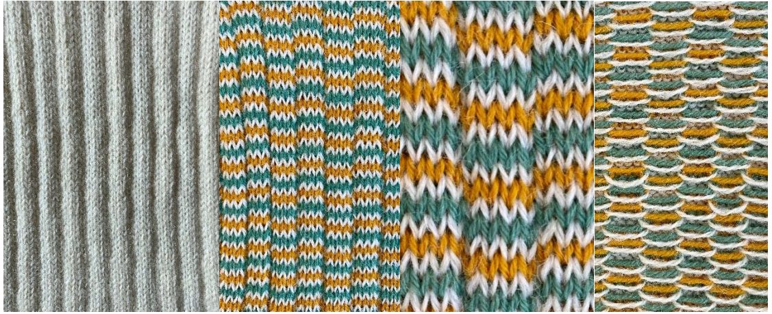
Figure 7:57 Sample 265 a 4x1 rib-look structure with three yarn types. KR/ ecru in feeder A. BFL/ WFW, turquoise/ mustard interchange through feeder B
