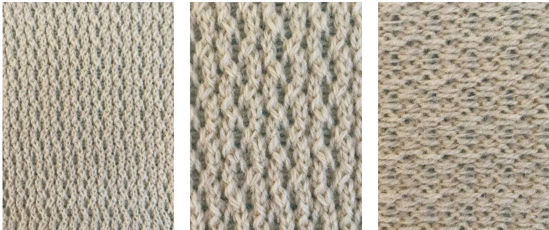
Figure 7:54 Sample 386 2x1 rib-look with pointelle in ecru combining three yarn types (DH, KR and BFL1).
