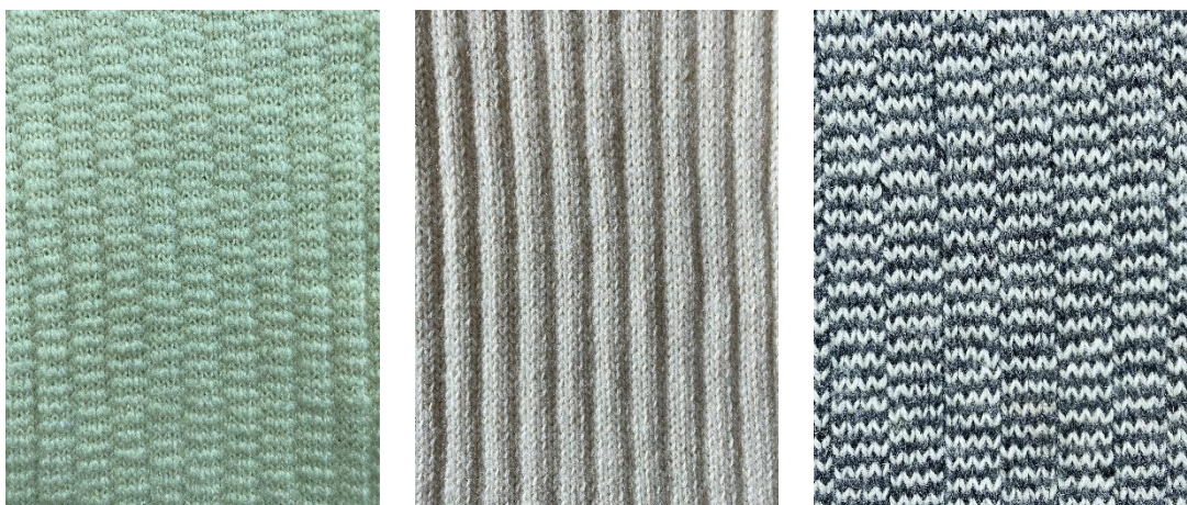
Figure 7:56 4x1 rib-look two yarn type structures in ecru and colour. Sample 139 (BFL1/ Southdown) and sample 137 (KR/BFL2).
