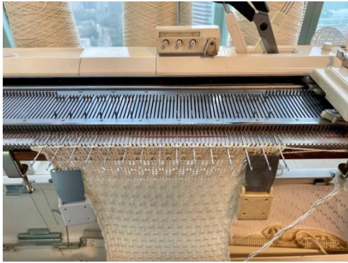
Figure 5:3 Step 2: Knit the body of the sample in the chosen pattern. Bind off the knit and take off the machine.
