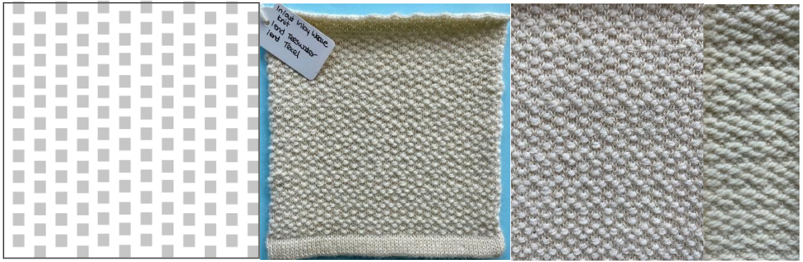
Figure 5:79 Sample 25 in/out Inlay in a 1x3 formation.
