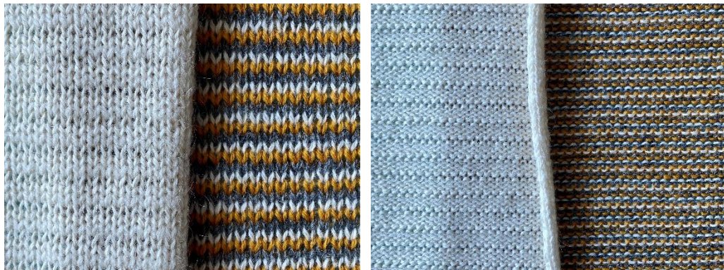
Figure 3:7 The face and reverse of a 1x1 (single course) knitted stripe structure knitted in three yarn types.
