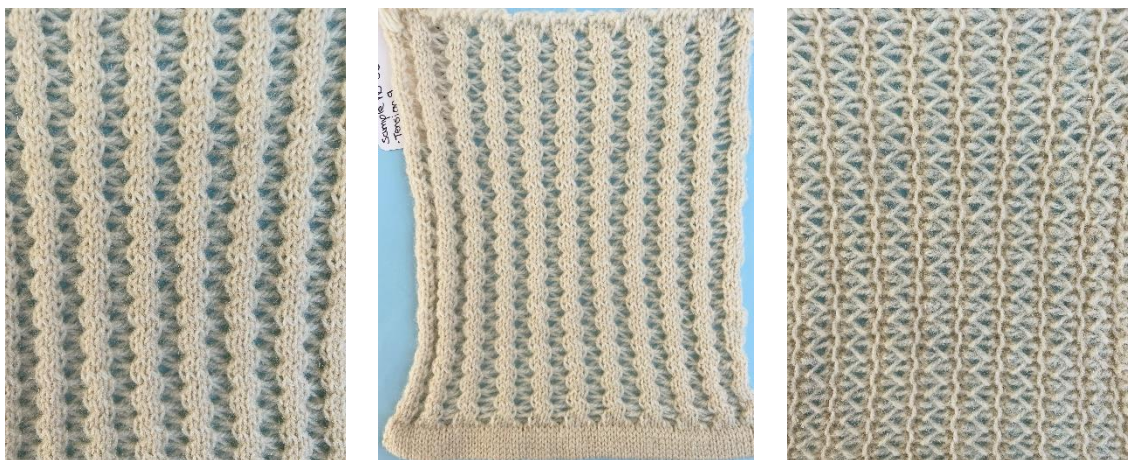
Figure 7:11 Sample 358, a 3x3 ladder structure manipulated with a racked look pick-up technique.
