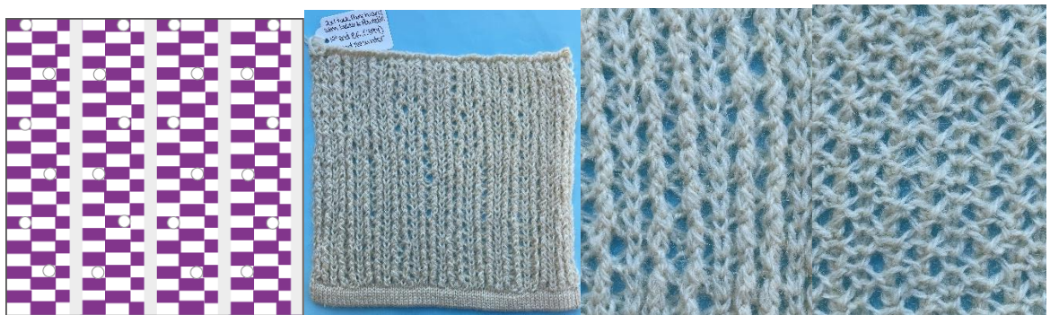
Figure 6:13 Sample 272 is a 2x1 rib look tuck jacquard structure with laddera & pointelle. This is the softest sample within the collection. The images show the front, back and a close-up of sample 272. (Image 6:15 is a bigger version of this sample). Samples 263 & 271 were knitted in the same structure.
