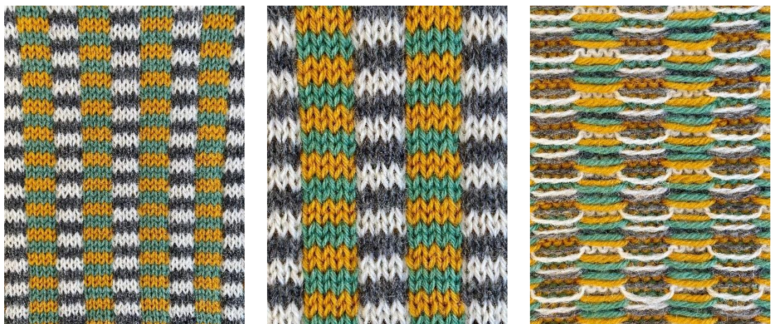
Figure 7:60 A 4x1 rib utilising four yarn types interchanging on every row.
