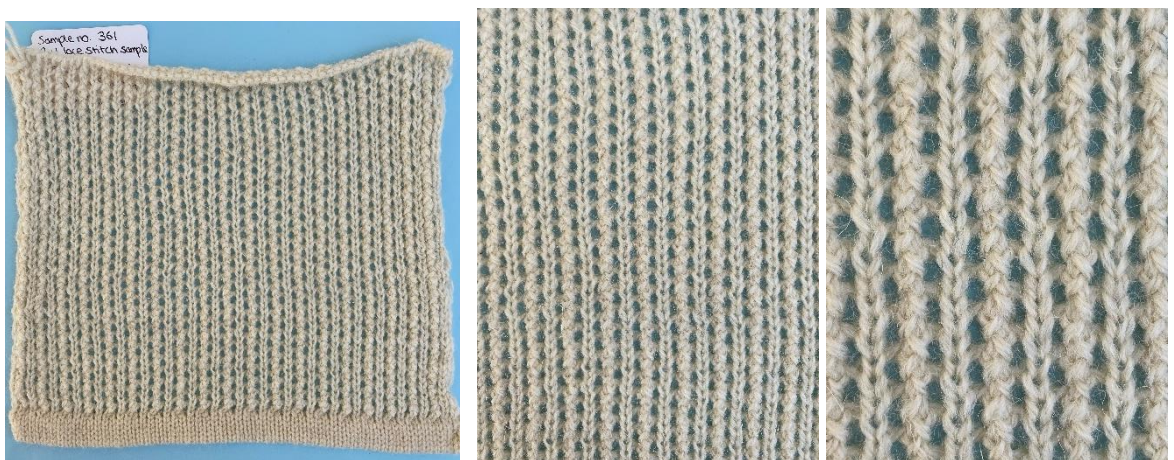
Figure 7:13 Sample 361 a 2x1 pointelle striped structure. (Two needles in action, one out, pointelle transfers on every row.)
