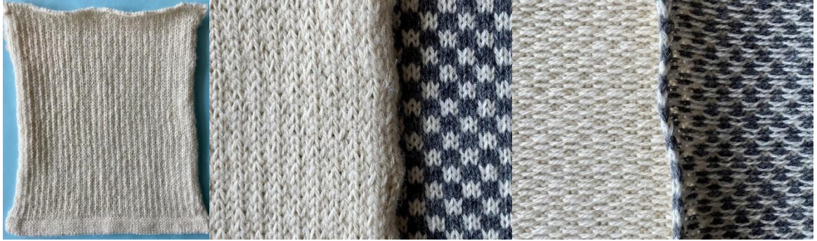
Figure 6:46 Details of sample 180. The images show the front and reverse of the fabric in ecru and colour to visualise how the yarns have been blended together.
