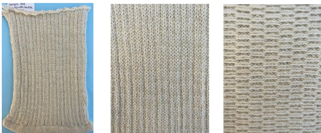
Figure 7:22 Sample 378, a 2x1 rib-look float jacquard with double ladder structure. The structure looks flatter than a 4x1 structure, but the floats on the back look similar. (4x1 structure below for comparison. Figure 7:23, sample 137.)
