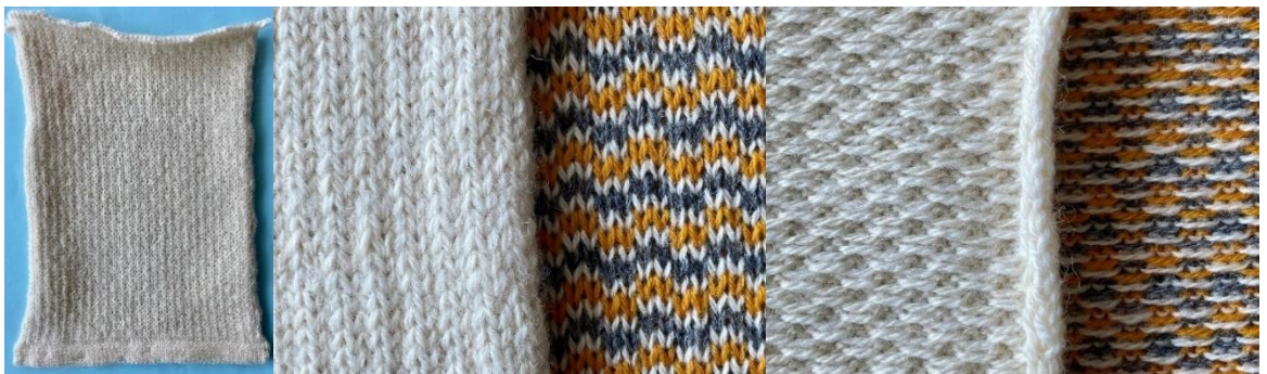
Figure 6:22 Details of sample 309, a 2x1 rib-look float jacquard structure. The images show the front and reverse of the swatch in ecru and colour to visualise how the yarns have combined.
